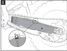
Mount the fork protection (B) framing it with the support (D) and hook the rubber band
