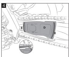
Place the support (D) identifying the anchor points, insert the zip ties (E) as shown in figure and close them.
