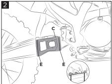
Place the support (C) and close the zip ties (E) identifying the anchor points.
