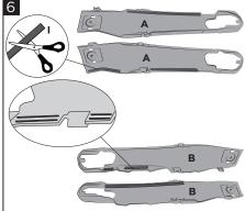
Recommended application: Cut the adhesive rubber strip (I) using the length of the various ribs as a reference and apply it to them on both covers.
