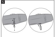
Insert the rubber band (F) in the dedicated space, as shown in figure on both protections.
